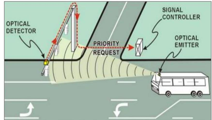
**Figure 9. A Typical Arrangement for Bus Priority Signals<sup>27</sup>**
