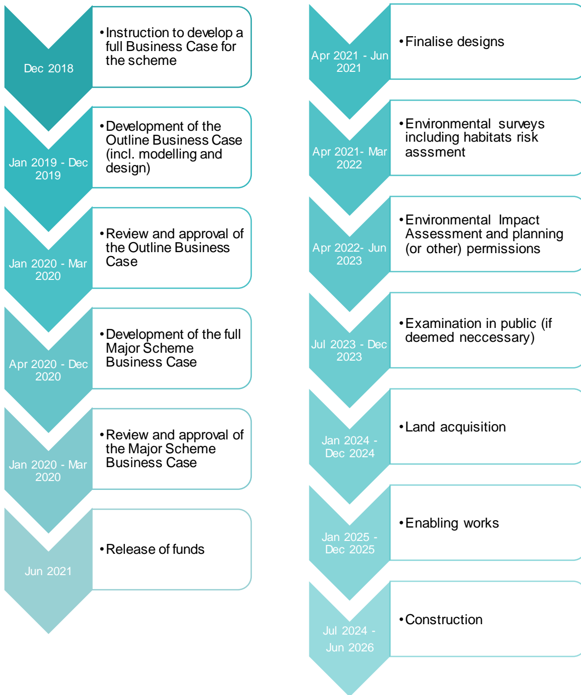
Figure 6.1: Indicative potential delivery programme for a link road between the M11 and the A47 based on traditional timelines and DfT guidelines
